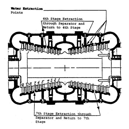
HP Turbine With Auxiliary Separators
