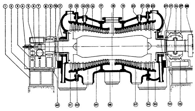
Typical HP Turbine with Extraction Steam after Stage 11
