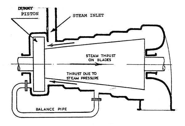
Single Flow Reaction Turbine with Dummy Piston
