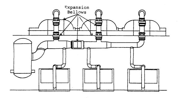
Expansion Joints on LP Turbine Inlet
