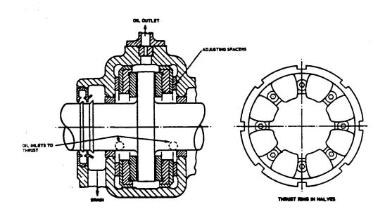
Tilting Shoe Thrust Bearing
